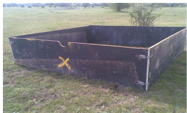
Form-ply sump showing latches
