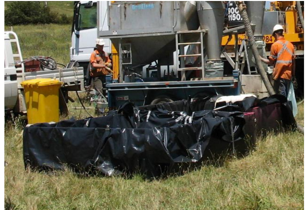
Sump set up at rig. Dust suppressor captures both sample and outside return in separate cyclones. Water is captured in bin beneath cyclones and drained into sump
